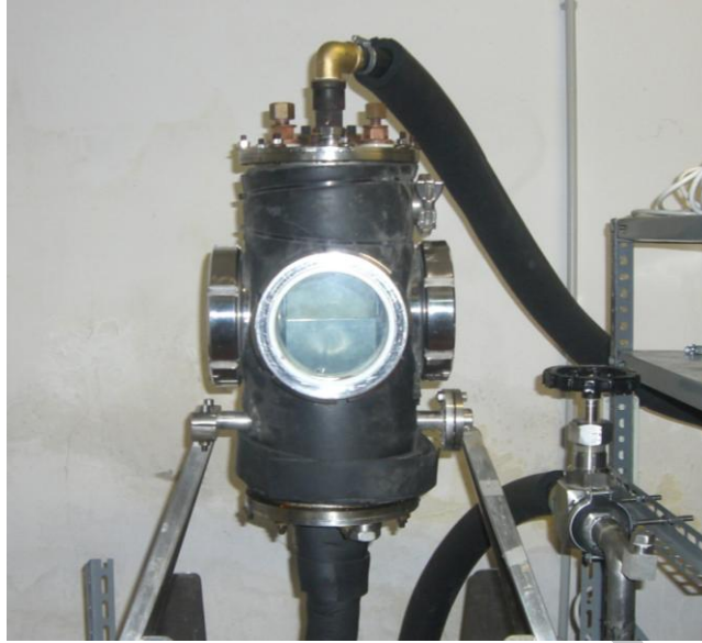
Figure 3: Picture of the test section, with inside the slot and the hydraulic and electric connections on the upper lid.
