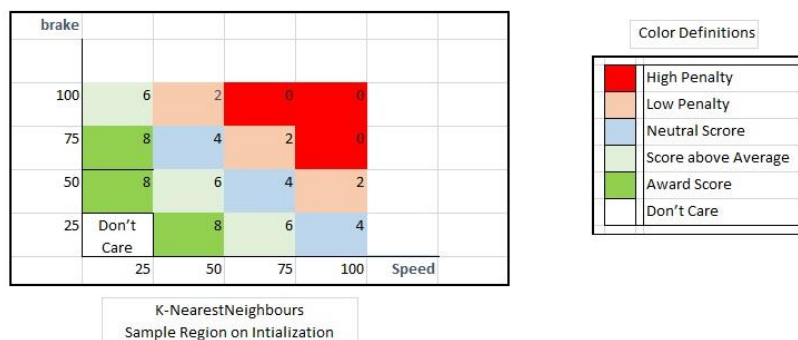
Fig. 6. Representation of the evaluation pattern of K-NN algorithm having multiple regions with different colors. The algorithm evaluates and maps the relativity between speed and harsh brake pattern. In case of high speed, if user applies harsh break, it will result in high penalty, which in turn will reduce the score.
