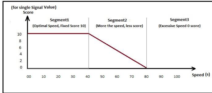
Fig. 7. Evaluation criterion for Linear Distances with representation of segments involving variation of speed signal values.
