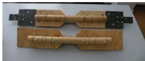
Figure 5. The specimen for traction tests on 3 rd type joint.
