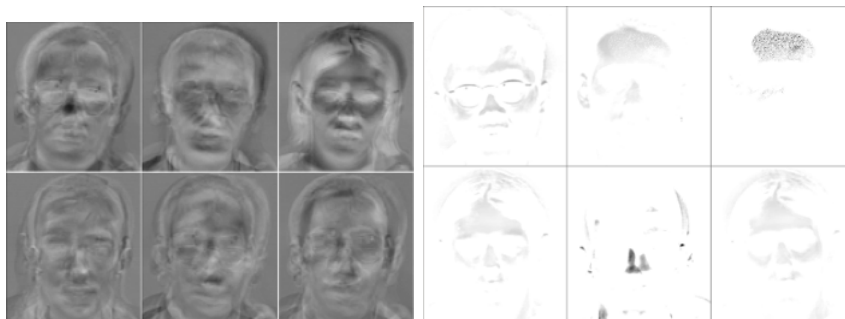
Figure 2.3: Comparison between bases extracted with PCA (left panel) and NMF (right panel).
