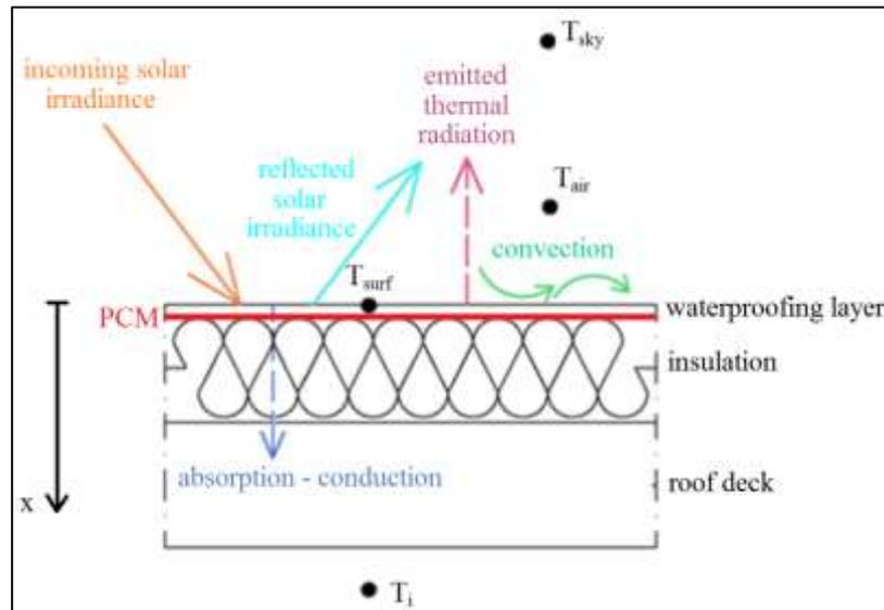
Figure 3. Roof structure and surface heat transfer processes.
