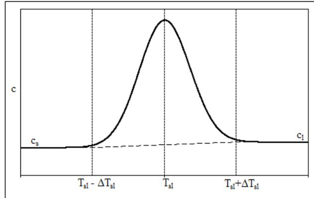
Figure 3. Effective specific heat of the PCM.
