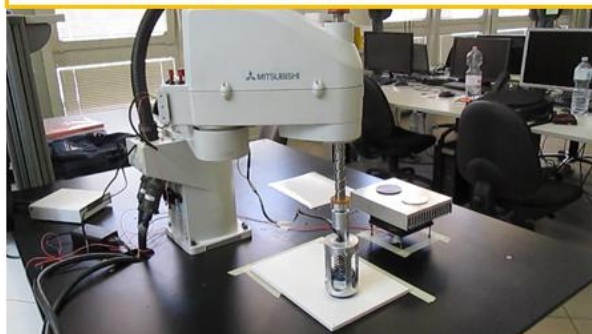
Figure 03. Positions of the emissometer head imposed by the robot.
