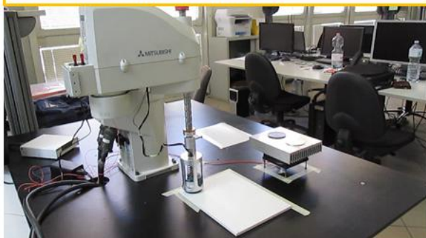
Figure 03. Positions of the emissometer head imposed by the robot.
