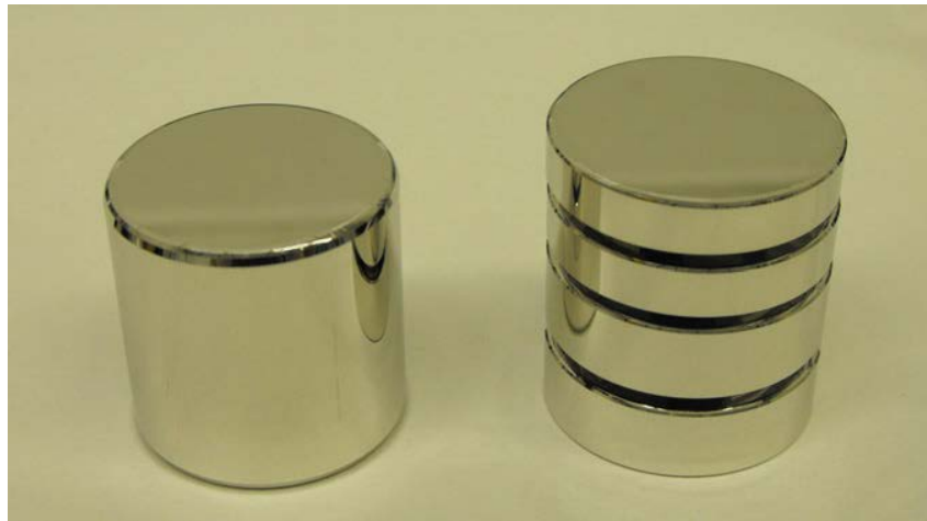
Figure 3. Integral and four piece sorption artefacts manufactured from platinum-iridium
