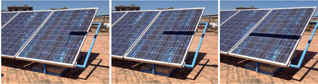
Fig. 7 Shaded panel. Case 1: the minimum shadow can vary from 225 to 450 cm 2 , (one or two cells covered); case 2: shadow varies from 450 to 900 cm 2 ; case 3 corresponds to the interruption of the panel.
