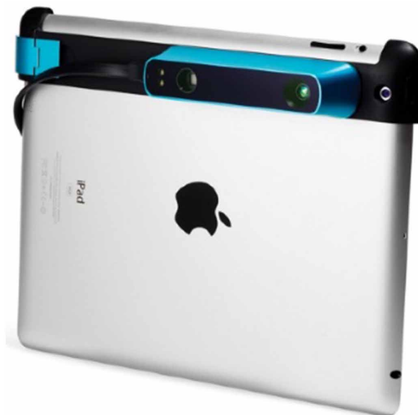
Figure 7. Structure Sensor clipped on the iPad
