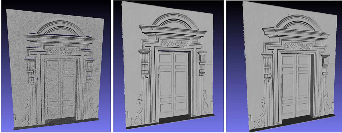
Figure 17. Mesh processing steps on the doorway: from the spikes meshes to the final smoothed model
