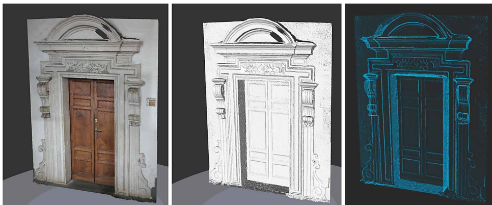
Figure 14. View of the overall doorway reconstructed by means of Image Based Modeling in different visualization modes: textured, shaded and x-ray
