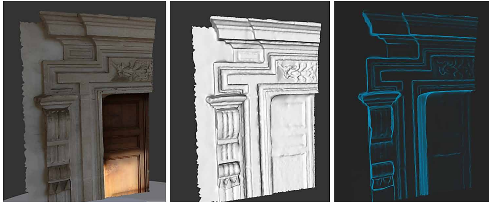
Figure 13. View of a detail of Image Based Reconstruction in different visualization modes: textured, shaded and x-ray
