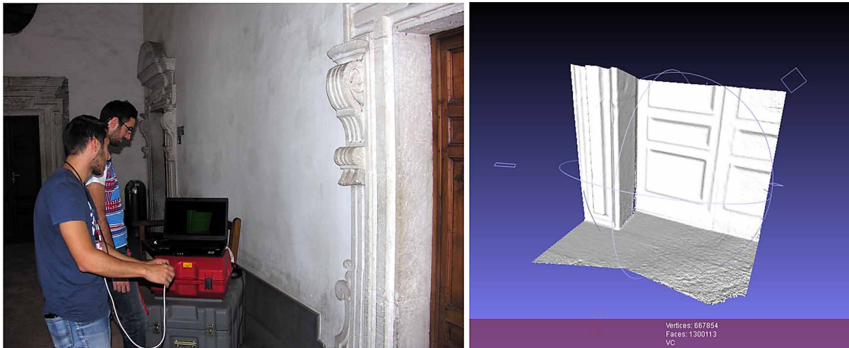
Figure 8. The bottom-left part of the doorway acquired through the Structure Sensor.
