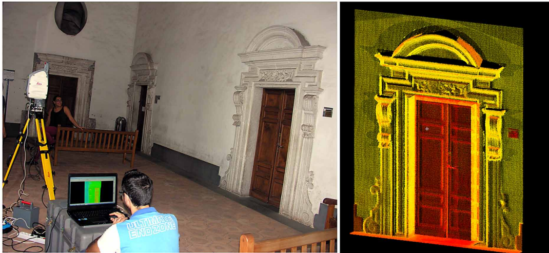
Figure 15. In situ 3D acquisition and view of the point cloud
