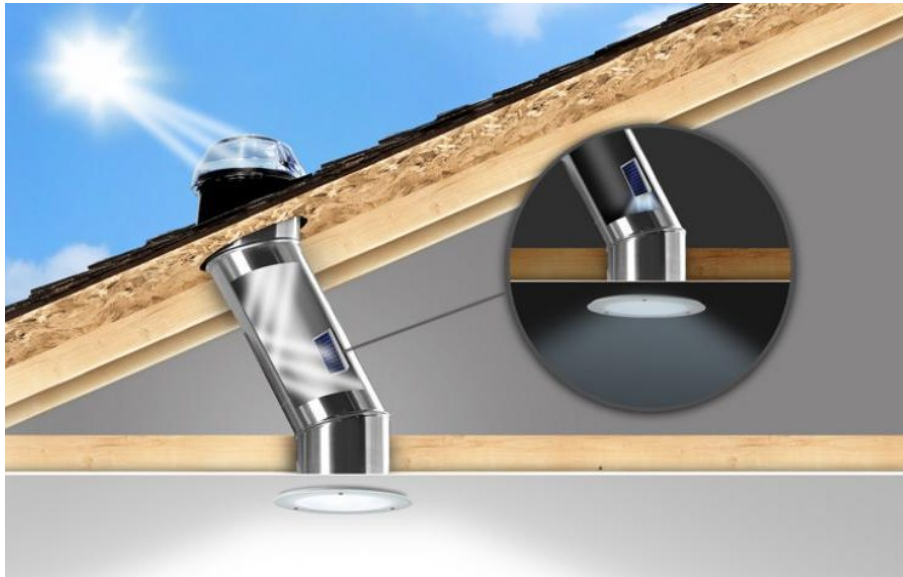
Figure 9. Scheme of a solar duct.
