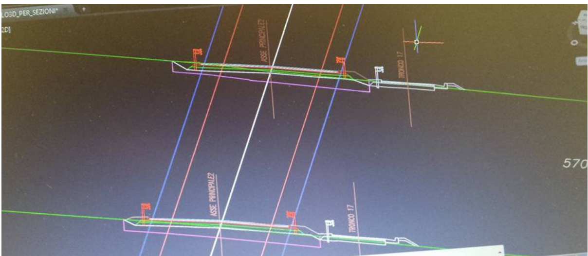
Fig. 84 Positioning of the rotated 2D road cross section on the road axis
