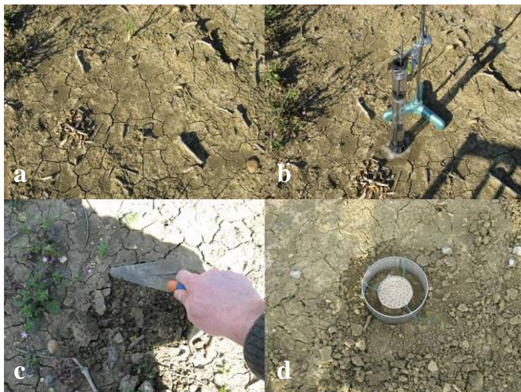
Fig. 1 Experimental procedure for determining the hydraulic resistance of the surface soil crust: a) surface crust; b) MDI experiment; c) crust removal; d) ring infiltration test.
