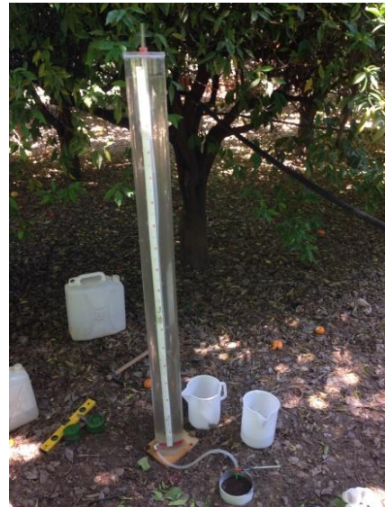
Fig. 1 Mariotte bottle used for the long duration infiltration runs
