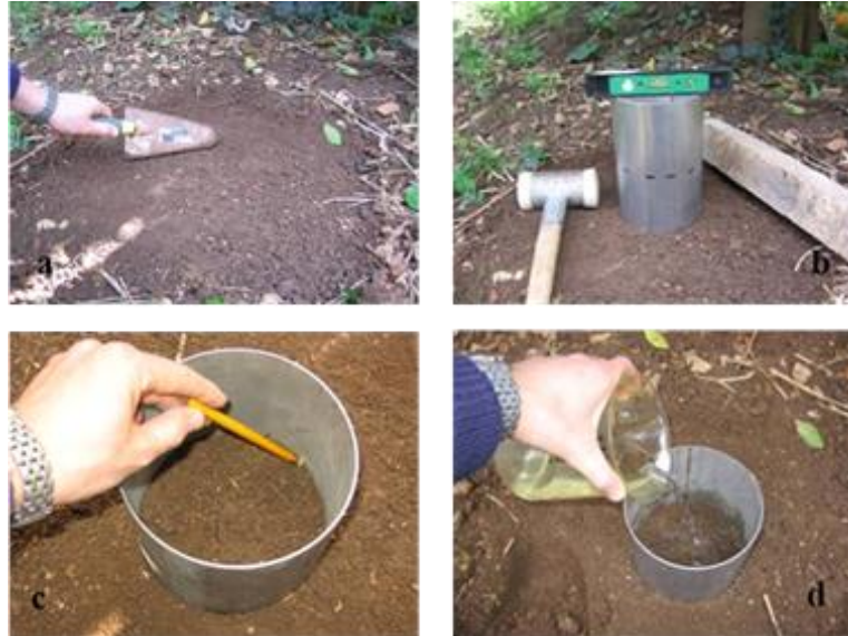
Fig. 2 Beerkan experiment: (a) removal surface vegetation, (b) ring inserted into the soil, (c) closing soil volume to inner wall sampler, (d) know water volume puring
