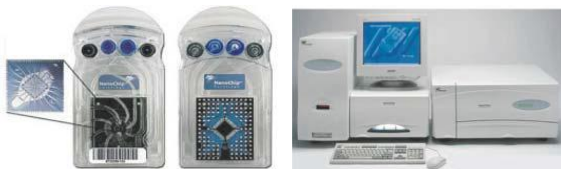
Figure 3.3: Photograph of the NanoChip® cartridge containing the electronic microarray (left), and Nanogen's Workstation which allows fully automated processing of 4 cartridges simultaneously in the loader and fluorescent detection in the reader (right) [62].
