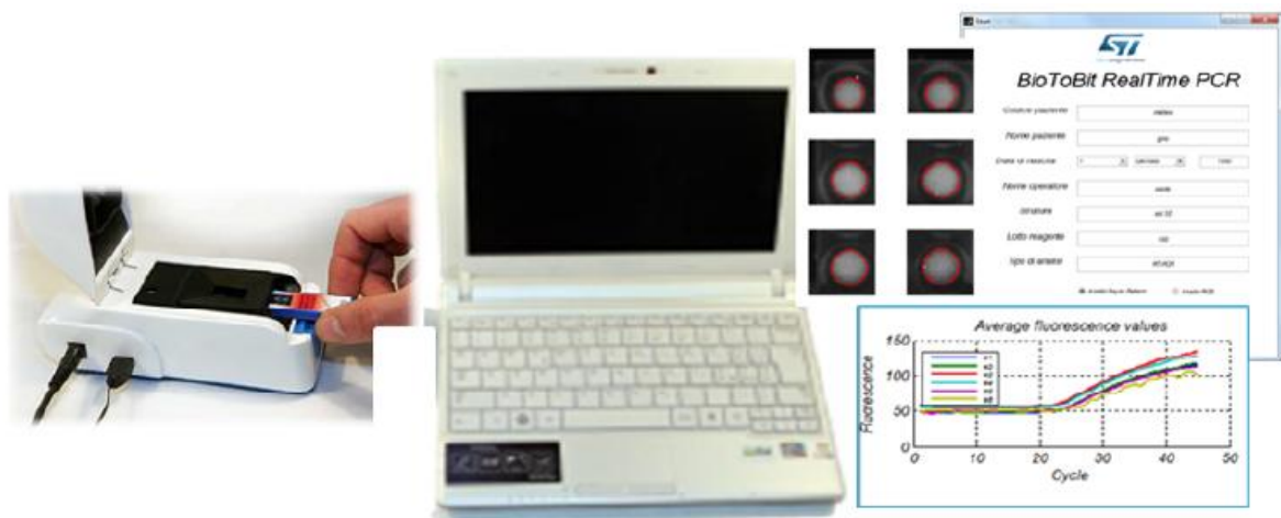
Figure 4.5: qRT PCR platform developed by STMicroelectronics [82].
