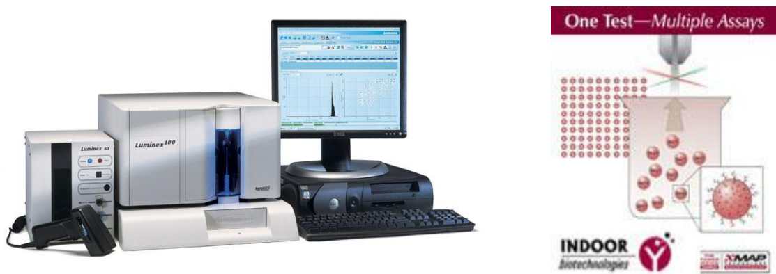
Figure 5. The Luminex machine: the microbeads are transported into the Luminex analyzer by using a precision sheath fluid stream to align them in single file, where they pass through two lasers, similarly to classical flow cytometry. The red laser excites the colours inside the microbeads to identify which microbead is currently being read. The green laser excites the colour on the microbead surface, i.e. the labeled reporter tag. Finally, the color signals are detected by an advanced optical system, and the signals are processed into data for each reaction.
