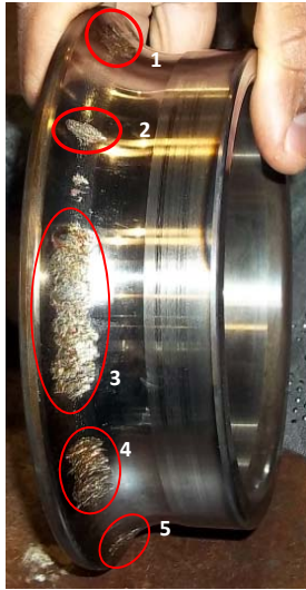
Figure 2.20: Bearing 7320BECBM (N°1) inner ring damaged
