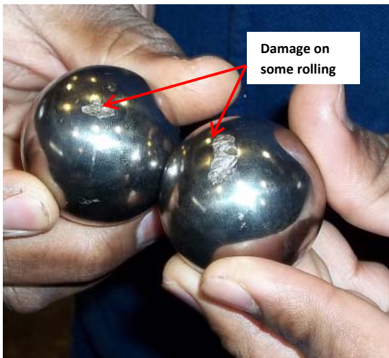
Figure 2.19: Bearing 7320BECBM (N°1) rolling elements (balls) damaged
