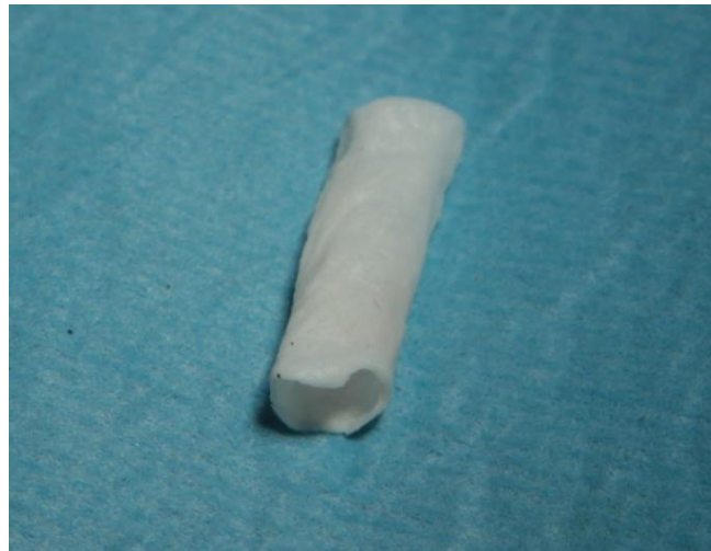
Figure 20. Tubular scaffold in PHEA-PLA+PCL
