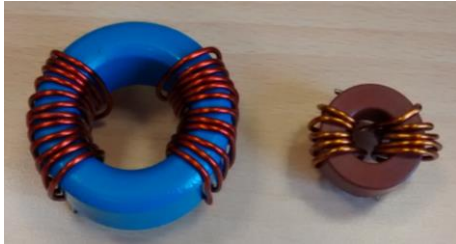
Fig. 9. CM choke set up by using an N30 ferrite core (left) and a VITROPERM core (right).
