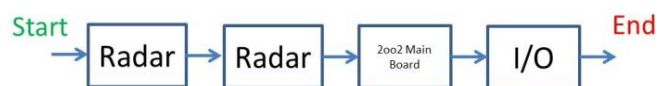
Figure 6. Reliability representation (RBD) of the proposed detection system based on radar sensing technology (case of two radar systems).
