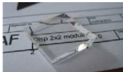
Fig. 3: One of the light guides designed for the focal surface of the ASTRI SST-2M prototype.
