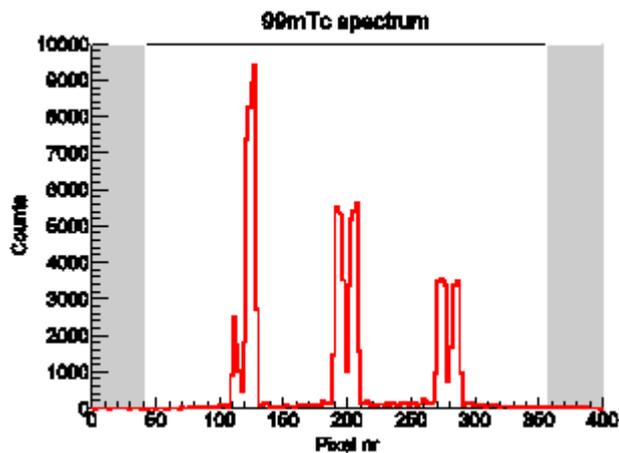
Fig. 2. Simulated output image of  $^{99m}\text{Tc}$  without the contribution of the other technetium isotopes.
