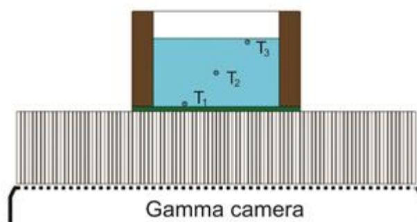
Fig. 1. A cross section sketch of the simulated water-filled container, with the capillary tubes placed on the parallel-hole collimator of the gamma camera positioned underneath. The colors represent the different materials, as defined in the Geant4 material database: water (cyan), air (white), steel (brown), glass (green) and lead of the collimator (dark gray). The capillary tubes with the fluctuating technetium solution are indicated as T<sub>1</sub>, T<sub>2</sub> and T<sub>3</sub>.
