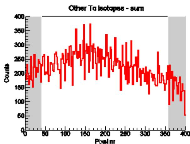
Fig. 3. Simulated output image of the total contribution of the technetium isotopes  $^{93}\text{Tc}$ ,  $^{94}\text{Tc}$ ,  $^{95}\text{Tc}$ ,  $^{95m}\text{Tc}$  and  $^{96}\text{Tc}$ .
