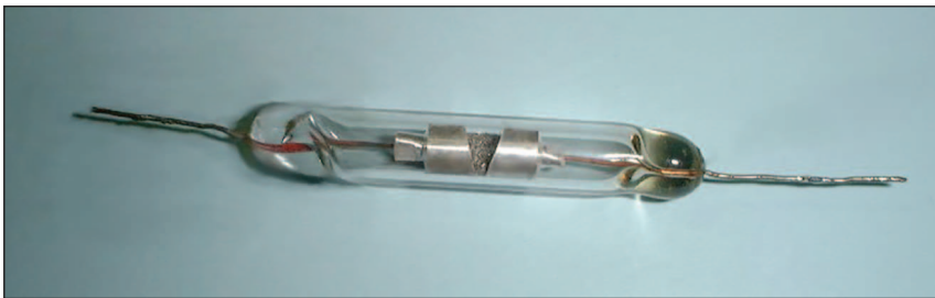
FIGURE 3 – A Marconi advanced filings coherer. (Photo courtesy of Wikimedia Commons.)
