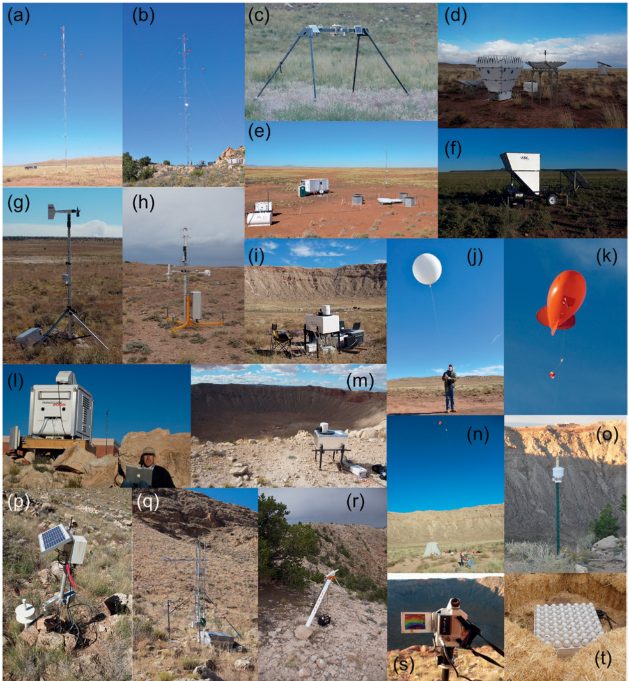
FIG. 4. Photographs of METCRAX II instrumentation. (a) 50-m tower at NEAR, (b) 40-m tower at RIM, (c) radiation balance station at FLR, (d) sodar at NEAR, (e) RWP-RASS at RWP, (f) sodar at FAR, (g),(h) surface weather stations, (i) lidar at the crater floor, (j) radiosonde, (k) tetheredsonde, (l) lidar at the north rim, (m) lidar at the east rim, (n) in-crater operations during IOPs, (o) HOBO temperature data-logger, (p) barometer on the inner crater sidewall, (q) sonic anemometer on the southwest crater sidewall, (r) scintillometer transmitter, (s) infrared camera, and (t) sodar downstream of the crater basin. The locations of the instruments are shown in Fig. 3.
