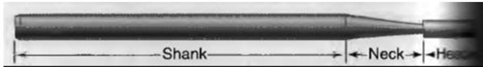
Picture 2. Normal designation of three parts of rotary cutting instruments.
