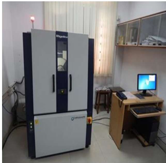
Figure 2.8: Multipurpose X-ray diffraction system (Rigaku ULTIMA IV)
