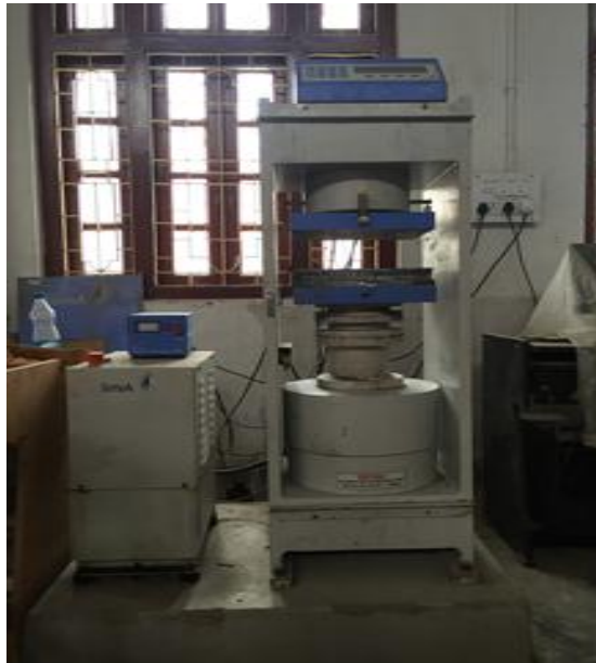
Figure 2.2: Compressive testing machine
