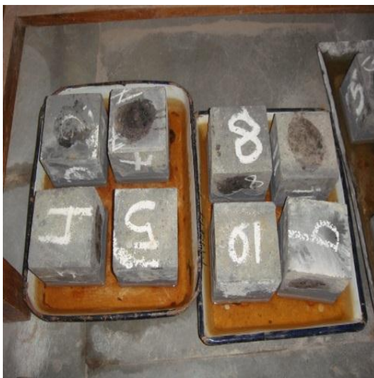
Figure 2.4: Capillary water absorption test set up
