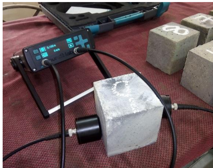
Figure 4.11: UPV test set up
