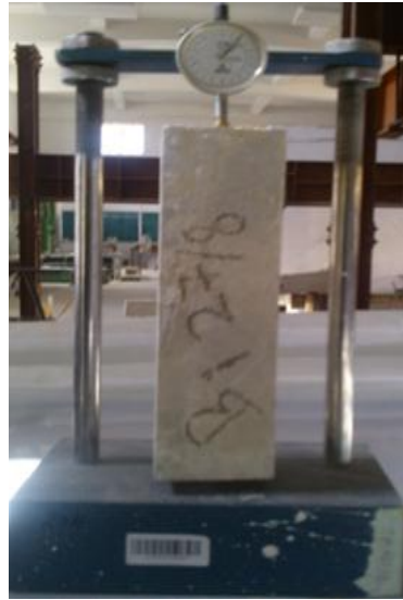
Figure 2.5: Drying shrinkage test
