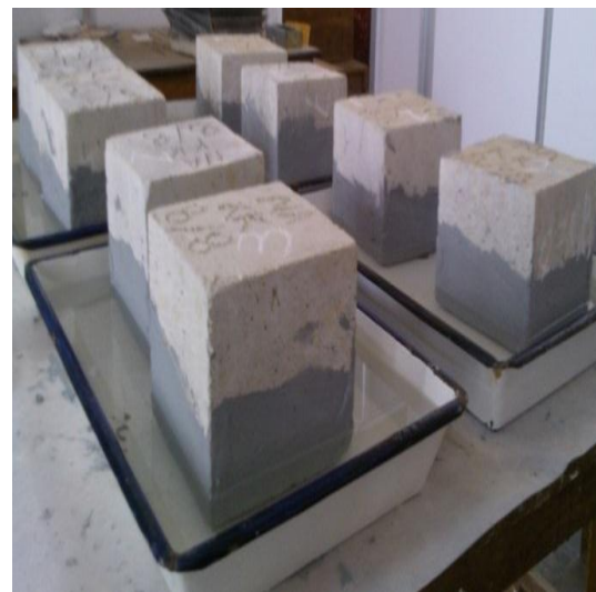
Figure 2.4: Capillary water absorption test set up
