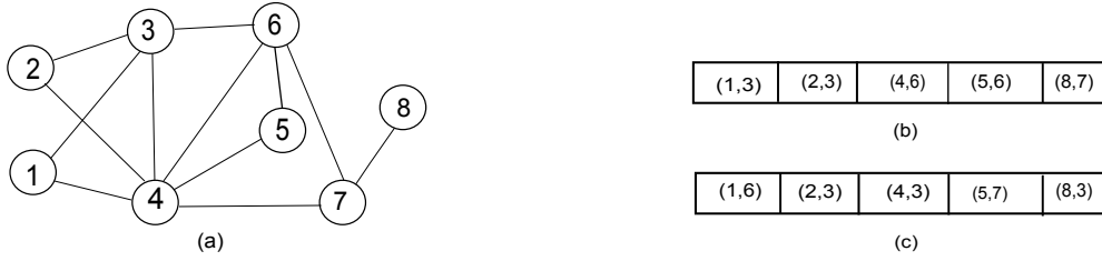
Figure 5.2: (a) WSN topology of 8 nodes, (b) Valid Chromosome, and (c) Invalid Chromosome
