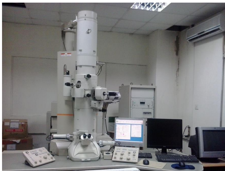
Fig. 2.8. Photograph of JEOL-JEM 2100 TEM.
