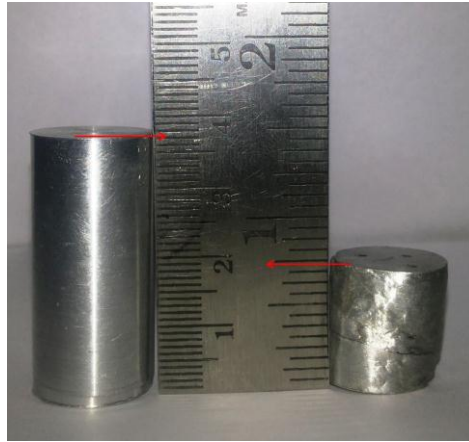
Figure 6.4: Compression test for determination of flow stress
