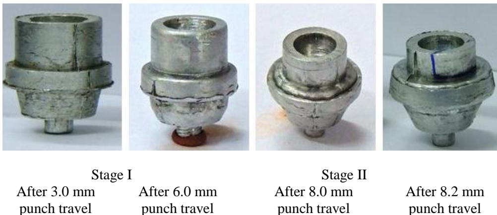
Figure 6.70: Die filling at different punch movement
