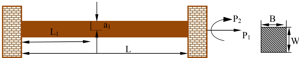
Figure 3.3: Geometry of the cracked fixed-fixed beam
