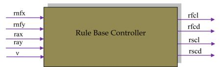
Figure 8.1: Rule base controller for identification of multiple cracks.
