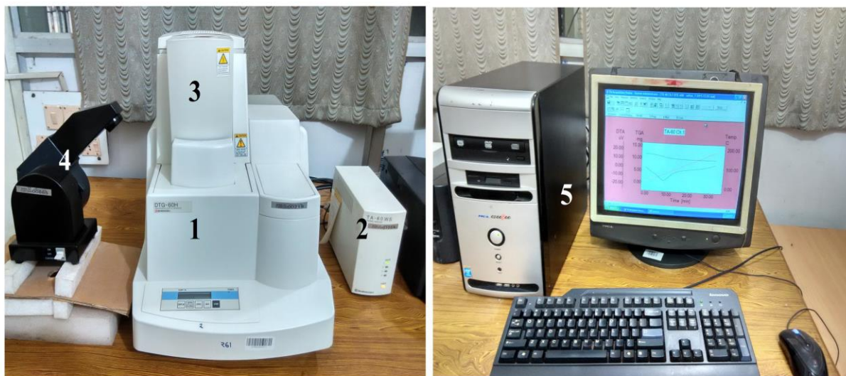
Fig 4.4 Photograph of the experimental setup of DTA
