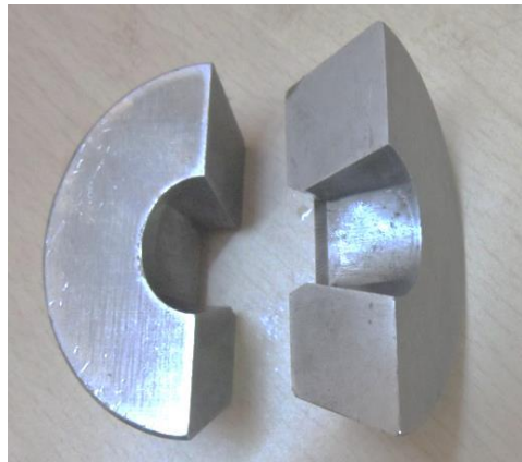
Figure 4.20: Linear converging round to square split die
