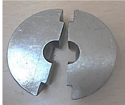
Figure 5.17: Cosine profiled split die
