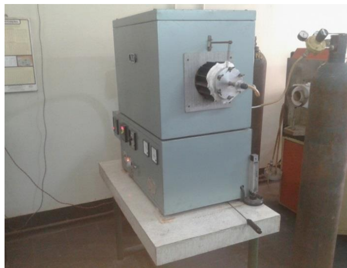
Figure 6.4: Controlled atmospheric furnace.
