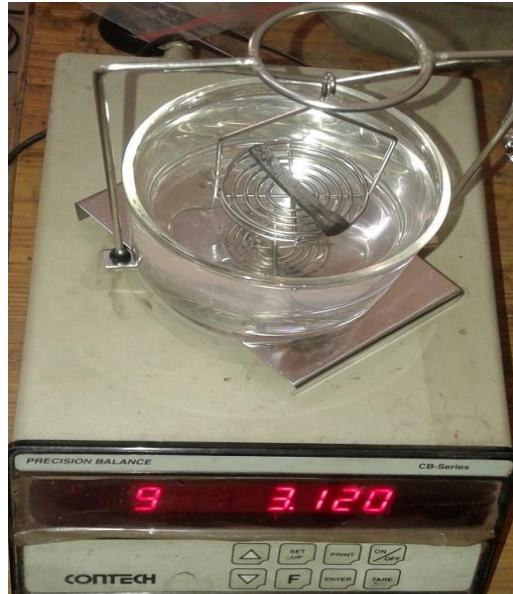
Figure 6.6: Density measurement kit with analytical balance.
