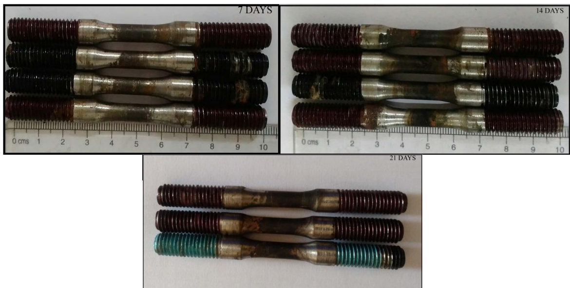
Fig. 4.7: Corroded samples of (a)7 days (b) 14 days (c) 21 days.
