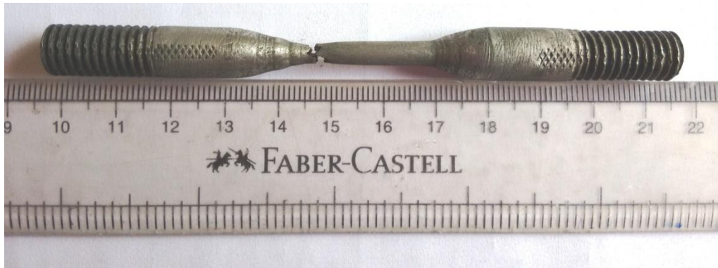
Fig. 3.4: Photograph of a broken post ratcheting tensile sample
