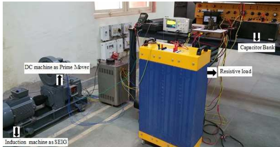
Figure 3.8: Experimental set up of SEIG system
