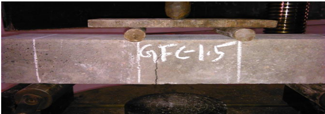
Fig. 4.5.3 Crack Pattern of GFC
