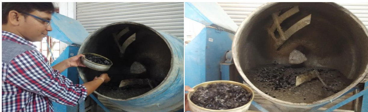
Fig. 3.3.1 Addition of Fiber to the SCC Mix
