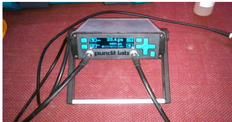
Fig. 3.2.6.4 UPV Test Set-up
