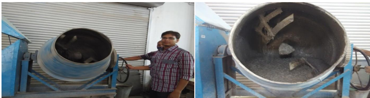
Fig.3.2.1 Concrete Mixture Machine & Preparation of SCC Mix
