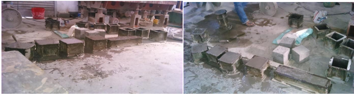
Fig. 3.2.4 Casting Of Specimens
