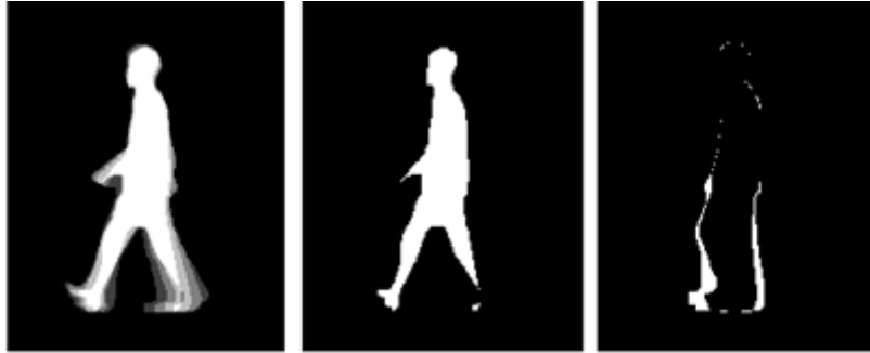
Fig. 2.4a – GEI, DEI and positive portion of frame difference
