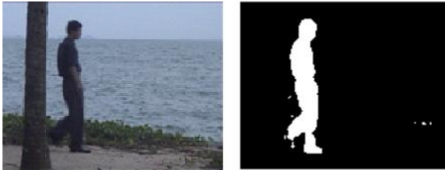
Fig. 2.1 – Sample result of fuzzy correlogram-based background subtraction method
