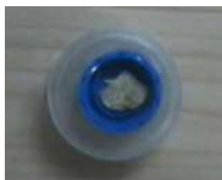
Figure 3.5 – Freeze dried porous scaffold with mould
