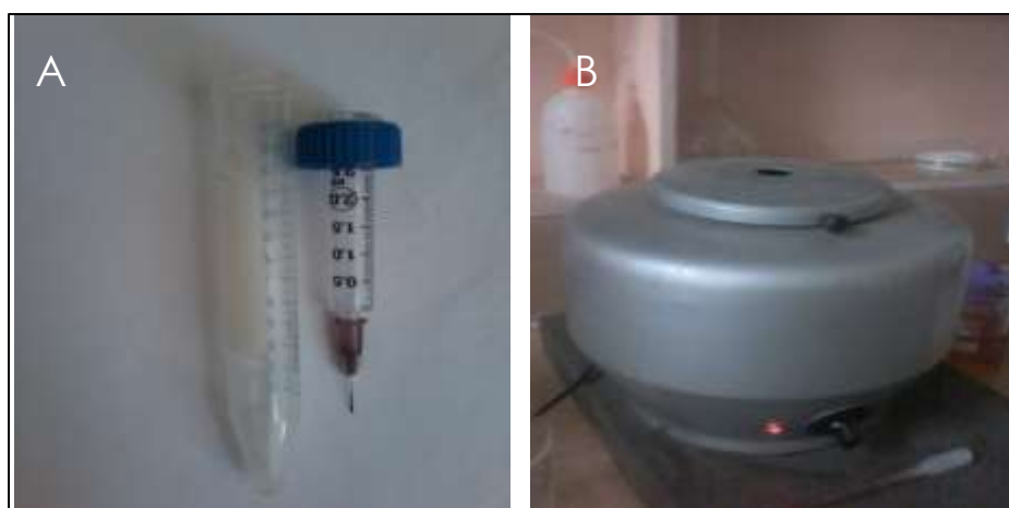
Figure 3.4 - A) Falcon tube with needle B) Bucket Centrifuge
