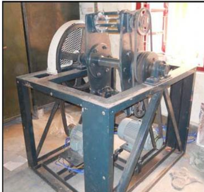
Fig. 4: Dual drive Planetary Ball Mill
