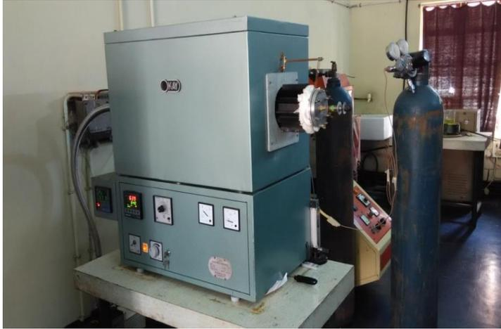
Fig. 3.4: Tubular furnace
