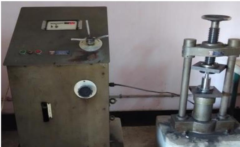
Fig. 3.2: Cold Uniaxial Pressing Machine
