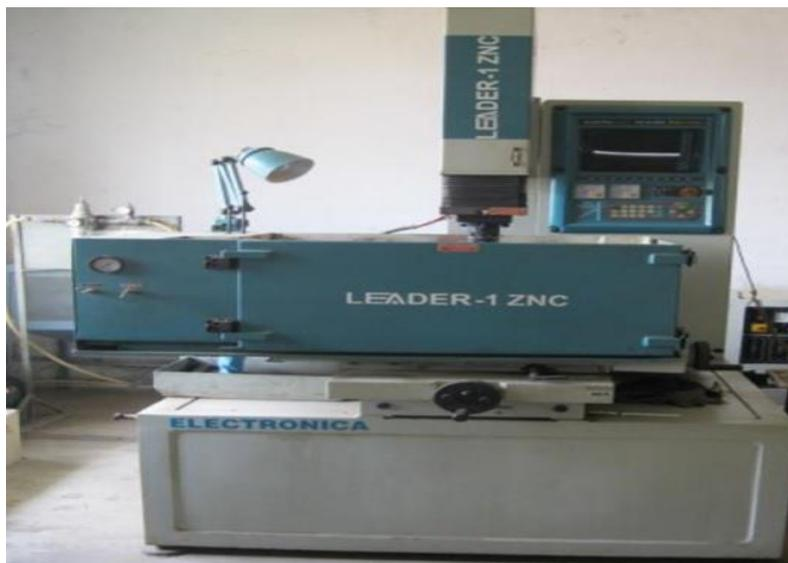
Fig. 3.6: Electro discharge machine
