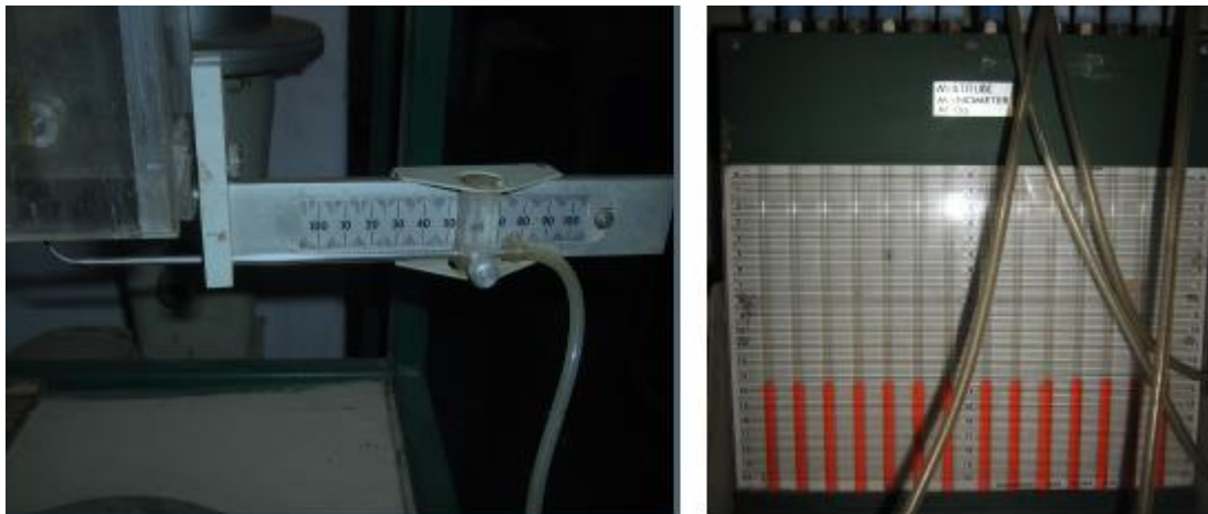
Fig 9. Test Apparatus (pitot tube , Multimeter Manometer)
