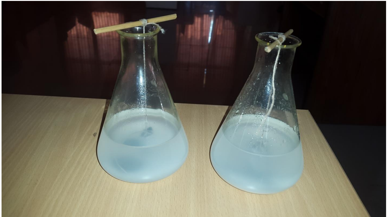
Fig. 3.9.2 Sample and solution after 24 hours of corrosion testing
