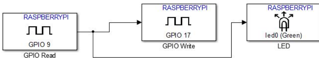
Figure 3- 8 Read from and write to a Raspberry Pi GPIO pin
