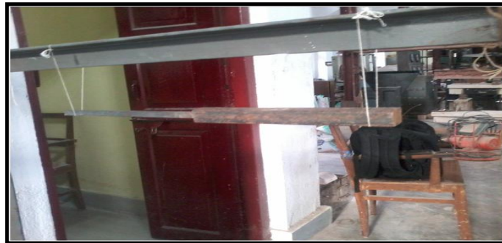
Figure 4.9 Vibration test setup for a stepped beam suspended through strings to look like free-free beam.
