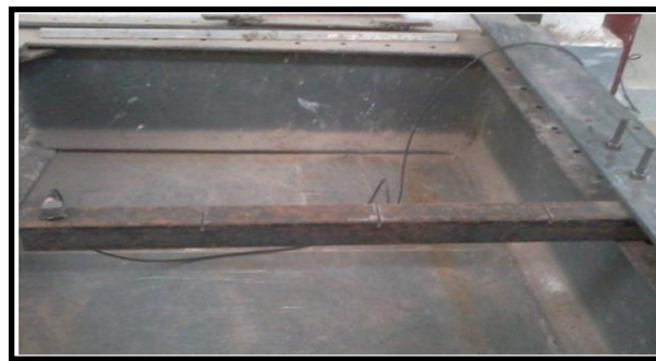
Figure 4.7 Vibration test setup for a cantilever beam with three cracks of uniform depth of 8mm present at x_1=125\text{mm} , x_2=250\text{mm} , x_3= 345\text{mm}
