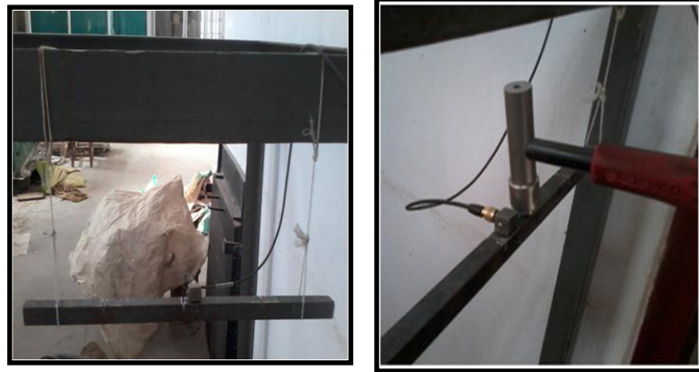
Figure 4.6 Free Vibration test setup, beam suspended by two strings like free-free beam, accelerometer and modal hammer in position
