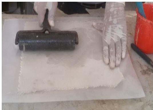
Fig.15: Steel roller is used to remove air
