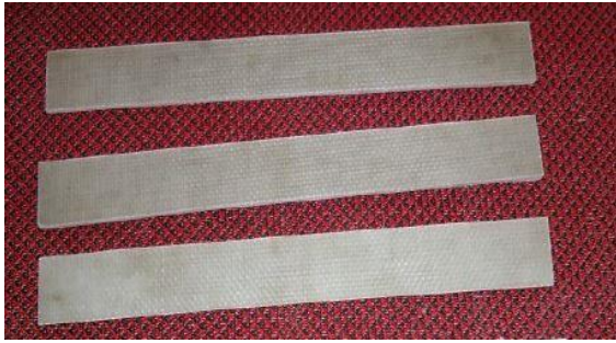
Fig.9: Laminated composite beam specimens for tensile testing.
