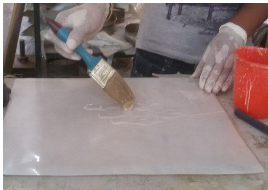
Fig.13: Resin is applied on plastic sheet
