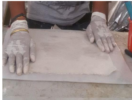
Fig.14: Woven glass fibre is laid on gel coat
