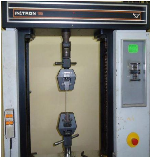
Fig.10: Experimental set up for tensile testing
