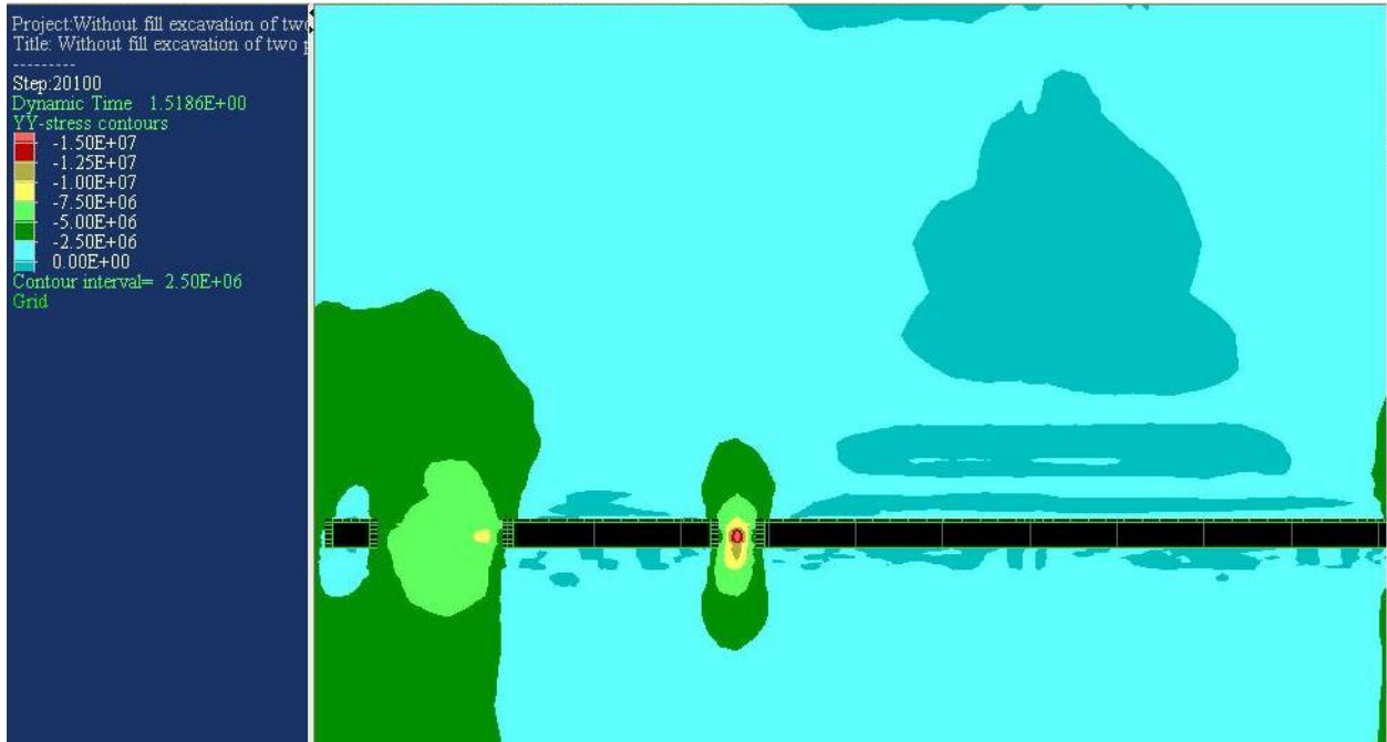
Figure 31: Stress distribution after extraction of two and half pillars with one rib
