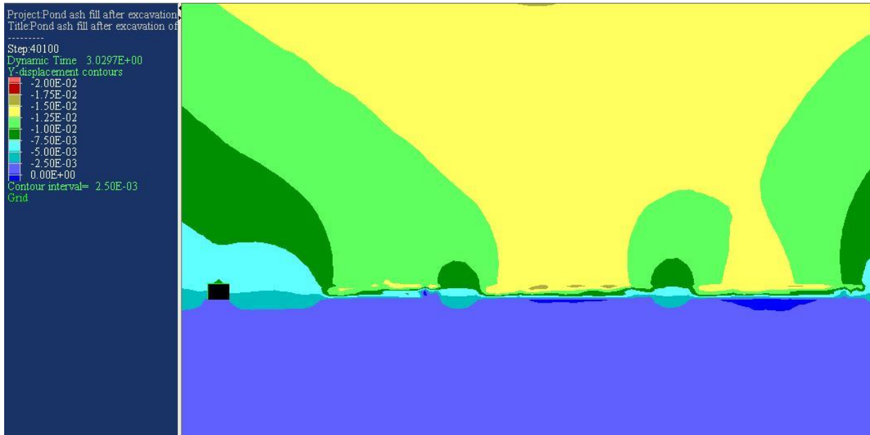
Figure 38: Displacement of the roof after excavation and backfilling of two and half pillar and one rib left with pond ash
