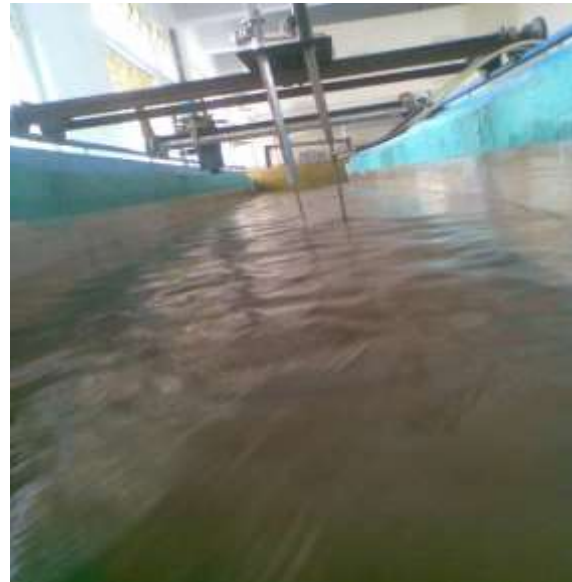
Fig.3.6 photo of the point gauge, pitot tube
