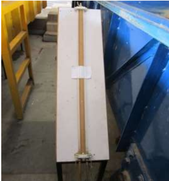
Fig.3.5 Photo of the inclined manometer used
