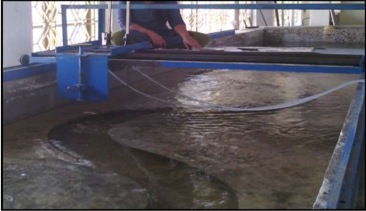
Fig.3.8: Moving Bridge Arrangement at the Bend Apex
