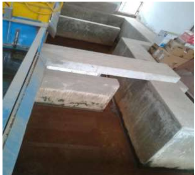
Fig.3.3: Photo of volumetric tank.
