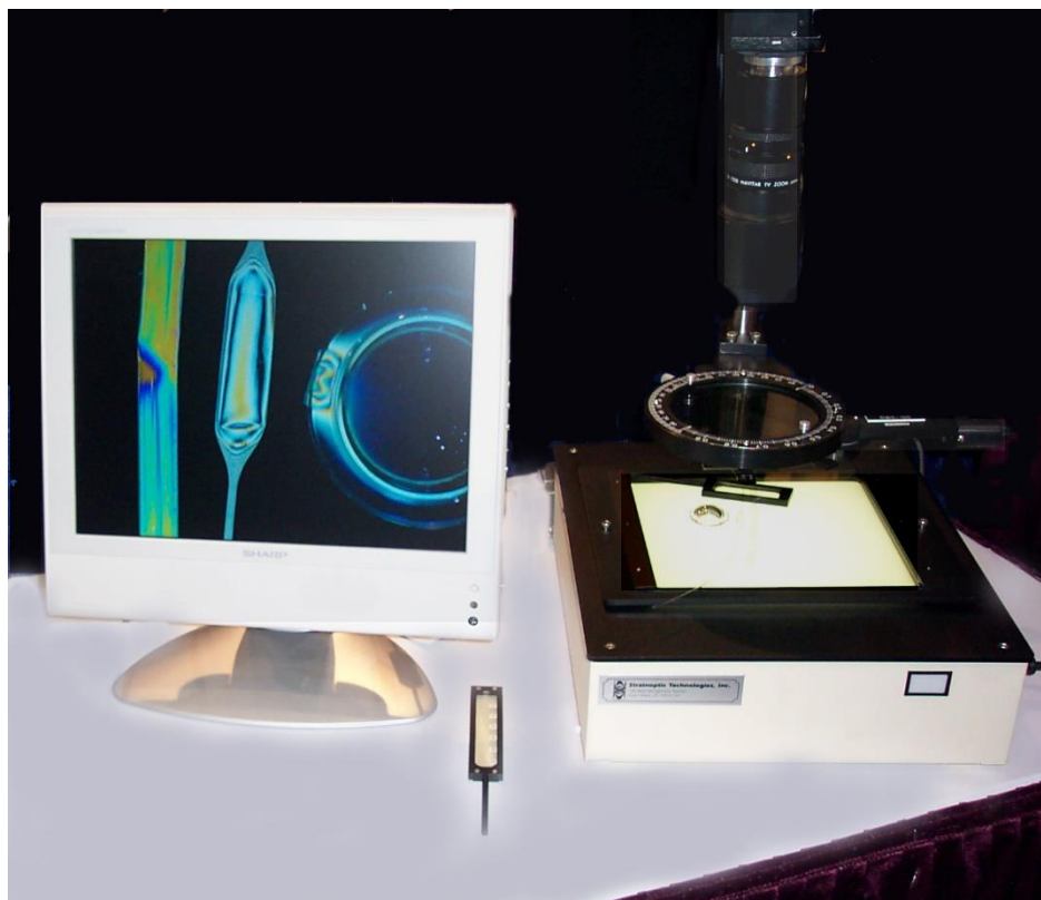
Fig. 4 – PS-100-SF Polarimeter, Strainoptics, INC. North Wales, PA 19454 USA
