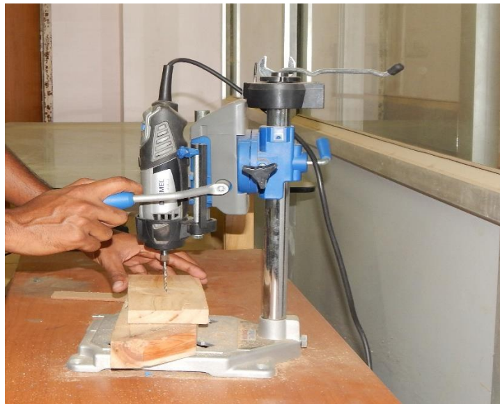
Fig: 3.14 Drilling holes for screw
