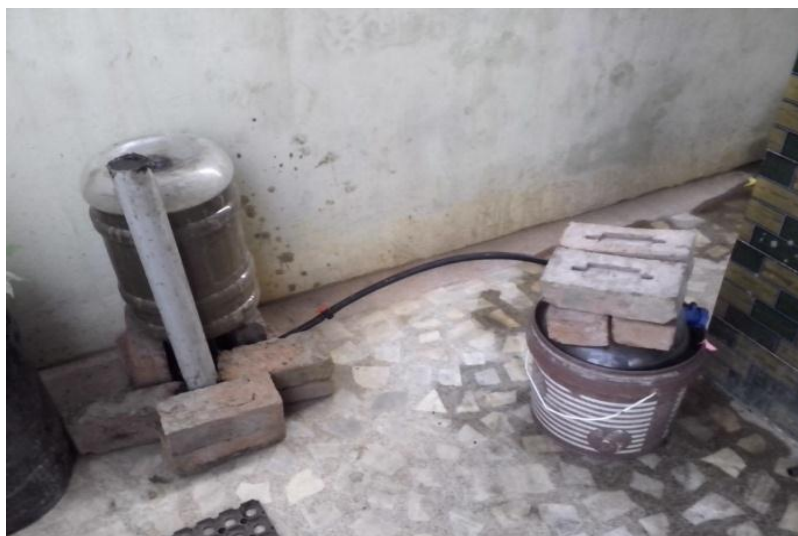
Fig. 4.2 20 L Digester experimental setup
