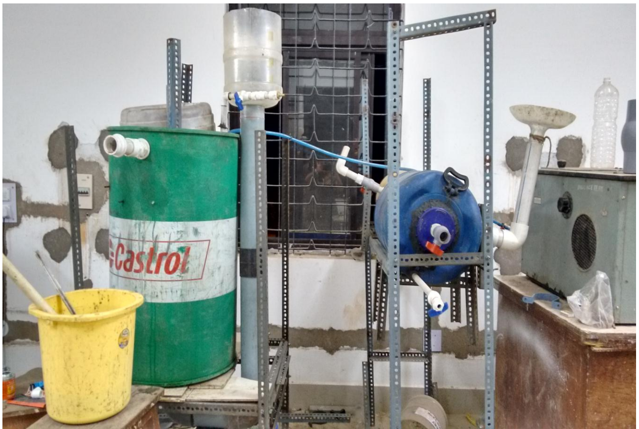
Fig. 6.2 Compartmental digester experimental setup
