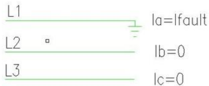
[Figure 2.1: Line to Ground Fault]
