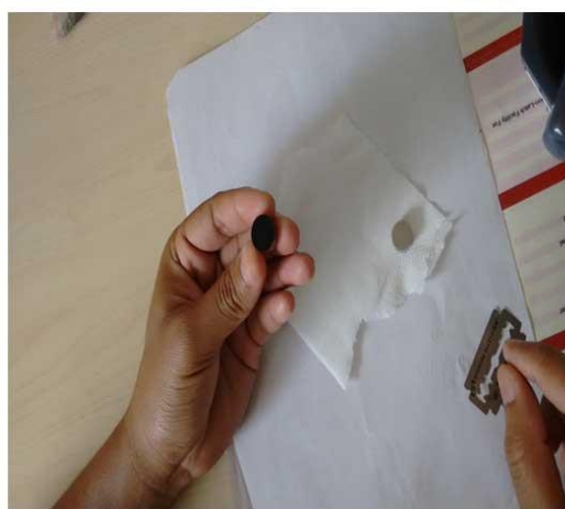
Fig.3.10 Pellet preparation before FTIR
