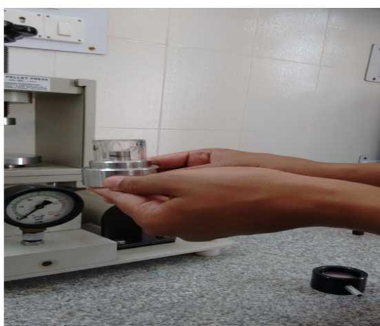
Fig.3.10 Pellet preparation before FTIR
